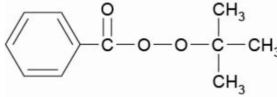
Organic peroxide used for curing unsaturated polyester resins, vinylester and acrylic resin at elevated and high temperatures; preferred for curing UP resin based Hot Press Moulding formulations (SMC, BMC, DMC etc.) in the temperature range of 120-170°C.
