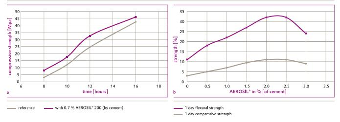
Addition of AEROSIL® fumed silica in concrete influences rheology of wet concrete strongly. It has a positive effect on homogeneity of component distribution within highly flowable concrete, such as self-compacting concrete (SCC). AEROSIL® fumed silica stabilizes SCC against sedimentation of coarse components during initial curing stages, it can reduce negative effects like "bleeding" (see **Figure 3**), etc.
