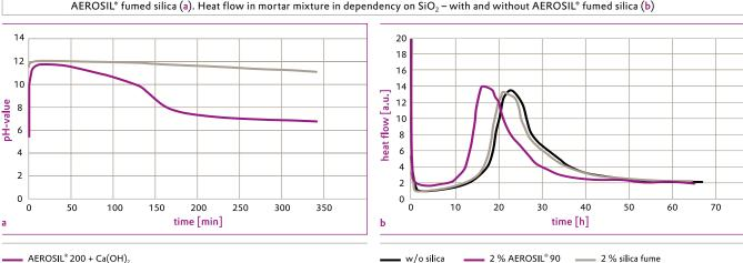
Figure 1 High pozzolanic activity of AEROSIL® fumed silica. Development of pH-value in SiO<sub>2</sub>-Ca(OH), mixtures with and without AEROSIL® fumed silica (a). Heat flow in mortar mixture in dependency on SiO2 – with and without AEROSIL® fumed silica (b)
