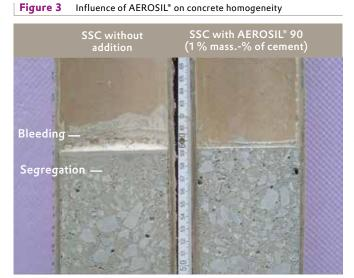
However, one should take into account, that use of AEROSIL<sup>®</sup> fumed silica grades with high specific area (AEROSIL<sup>®</sup> 200, AEROSIL<sup>®</sup> 300) increases the viscosity of wet concrete. If viscosity increase has to be limited, AEROSIL<sup>®</sup> grades with surface area about 100 m<sup>2</sup>/g, for example, AEROSIL<sup>®</sup> 90 should be used.
